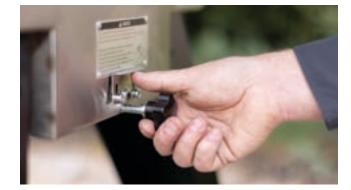
4. Replace ash cup and close the ash clean-out by pushing the knob back in and securing it under the locking collar.
