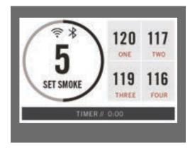
A smoke setting of 1 will produce less smoke and maintain a more even temperature. As the smoke setting increases, the temperature fluctuations will also increase.
