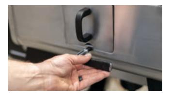
3. Rotate the valve handle to the horizontal position to allow flames into the smoke box. Once the wood/charcoal has started, rotate the valve handle back to the vertical position to smoke.
