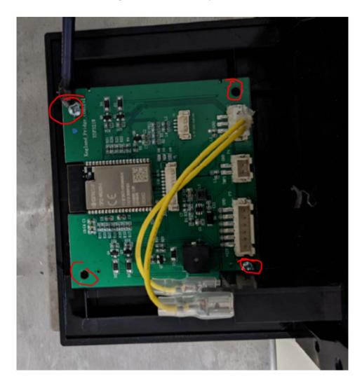
If you are replacing the screen PCB board with a new one make sure to remember to remove the protective film before putting the new board into position:
