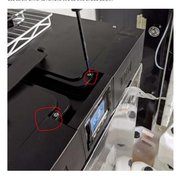
Remove screws from the underside of the screen as shown here:
