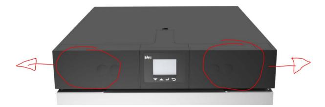
Slide the screen down so you can see the cables behind the screen:
