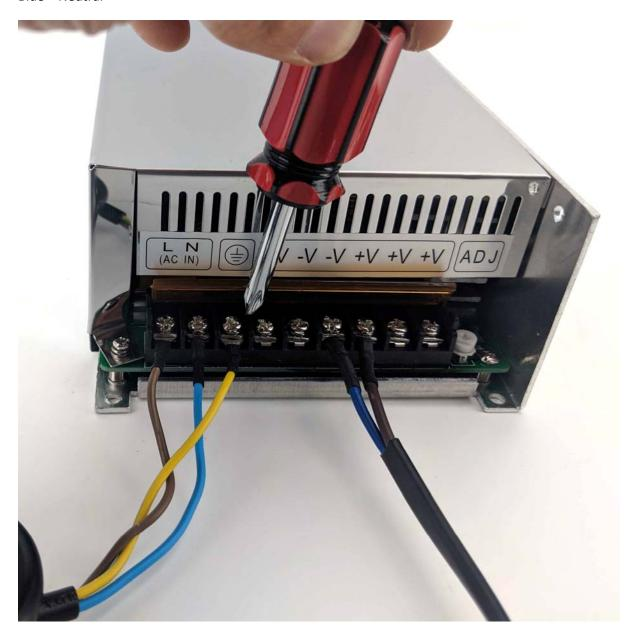
Use a Phillips head screw driver to connect the yellow/green wire to the earth terminal, connect the blue wire to the "N" (neutral terminal), and connect the brown wire to the "L" (live terminal).
