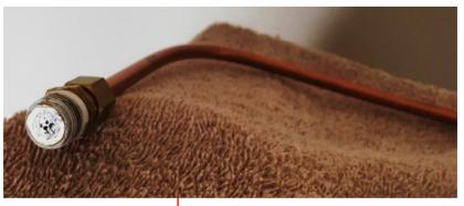
Very carefully clean out the tiny hole with a needle. DO NOT MAKE IT BIGGER, just gently clean it
