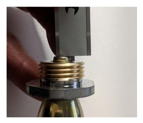
Ensure that the bulb protrudes from the bushing by at least 2mm.
