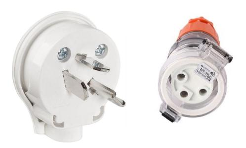
The plug on the left is the standard type that comes included with the brewery out of the box. This single phase plug is also commonly used for electric ovens or electric hob cooktops that you often see in your kitchen. Generally speaking the wiring for this type of plug will be 6mm<sup>2</sup> copper cable but we recommend you seek separate advice from your electrician to install suitable cable.
