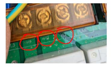
These three terminals are connected to the three active sides of the three heating elements.
