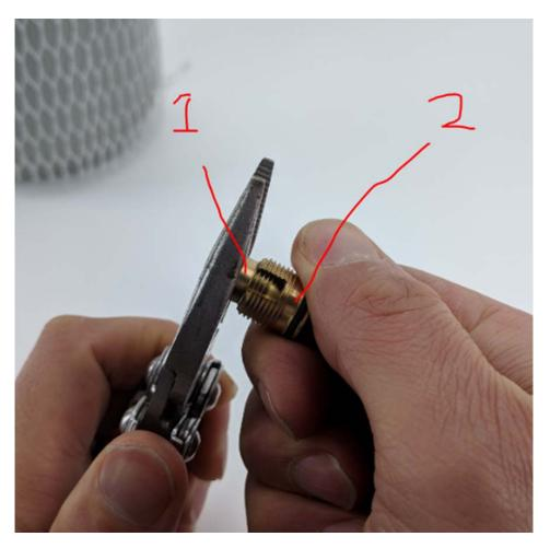
Now gas should be able to flow out of the RPV device freely.
