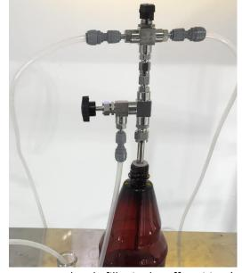
**Step 5.** Start with the handle of the counter pressure bottle filler in the off position (perpendicular to the unit).
