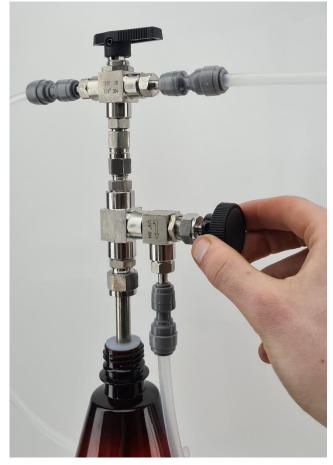
Step 8. After the bottle has been purged of any oxygen, close the bleed valve and pressurise the bottle back up to 10psi with CO<sub>2</sub>.
