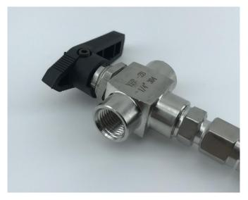
This leaves a ¼" female thread which suits a range of other fittings, however, the most useful of which is to install a liquid and gas ball lock posts with ¼ inch BSP bulkhead assembly (KL03179 and KL03162). This allows the counter pressure bottle filler to be quickly connected and disconnected from your existing kegging system.
