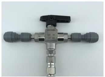
Ensure your hose has a clean straight cut with no burs, this can be achieved easily with a sharp Stanley knife or two in one tube cutter. Do not cute the hose at an angle. Then push your EVABarrier hose into the duotight fitting ensuring a good connection has been formed by gentling pulling back on the hose.
