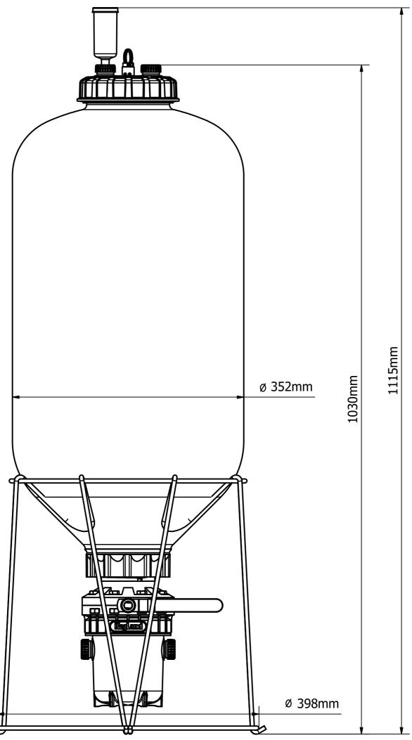
NOTE: The dimensions are of vessel not under pressure.
