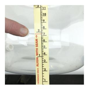
2. Stick the Stick-On Thermometer onto the outside of the fermenter. We suggest putting it next to the volume markings between the 10L and 20L markings.
