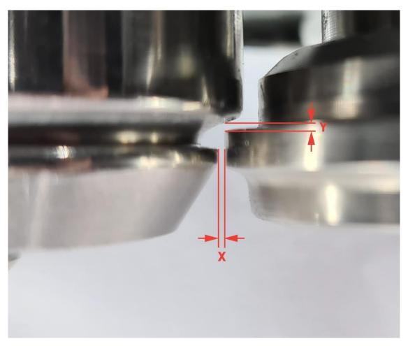
Note: The above photo is for demonstration purposes only. The 1<sup>st</sup> Op roller should be as close as possible (without touching) to the chuck in the Y direction.
