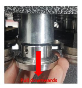
Then push the CDLE/CDL chuck as high as possible onto the drive shaft and retighten the grub screws to hold it in position.
