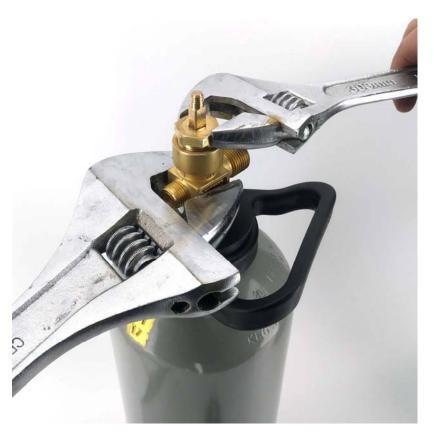
Step 4 Remove the valve core and stem.
