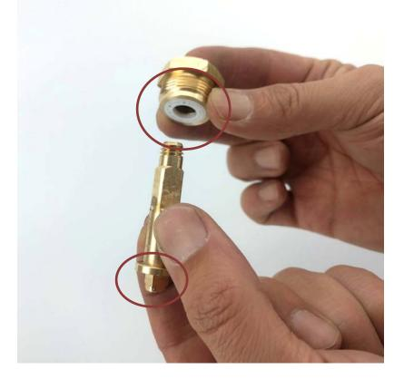
As shown above. Examine the valve stem. If the square drive on the end of the valve stem has worn down this may cause the handle to spin freely. If this is the case the valve stem needs to be replaced.
