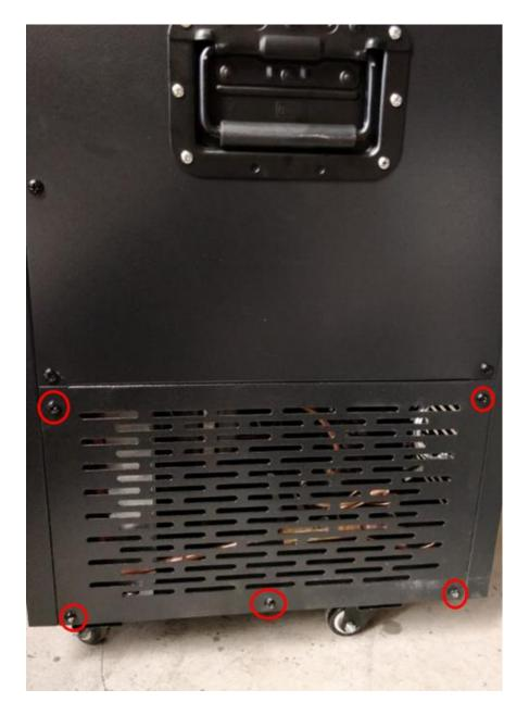
Step 1: Remove the 5 bolts holding the lower side wall.
