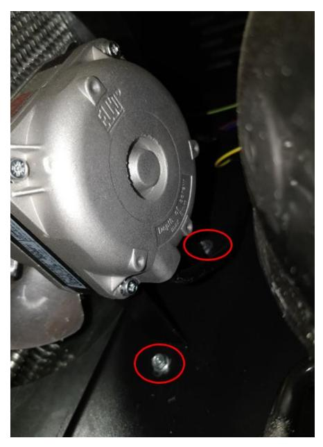
Step 4: Remove the x2 fan mounting bracket bolts.
