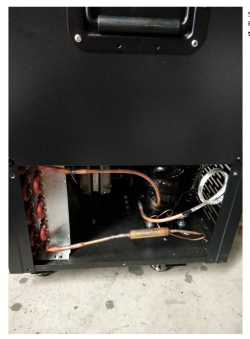
Step 2: Remove the side plate and sit it to the side.
