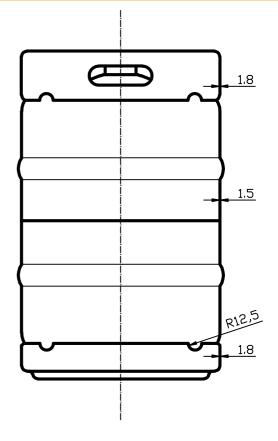
These kegs made in compliance with Australian Standards (AS2971) are manufactured with sanitary welds from 304 stainless steel. The kegs have nominal volume of 50L with total volume being 50.2L (±0.2litres)
