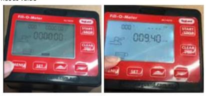
2. Press SET for 3 seconds and use the up and down arrows to set the pin number to 1234 (default password)
