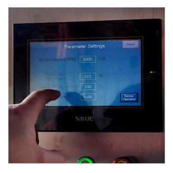
**3.2** – If you have adjusted from a 500mL Can you will need to increase the Timer Settings of the first Can Raise Delay or else the First Operation roller will start to engage before the can is fully engaged with the chuck.
