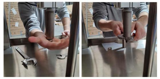
**2.6.6** – Once the can feels firm and in place, rotate the Bump Stop Shaft upwards until it touches the piston block. Followed by the locking nut. Then use the two spanners again to tighten against each other.
