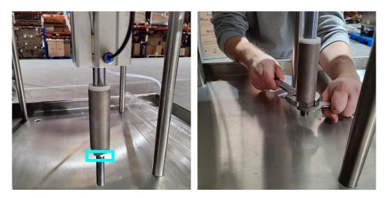
**2.6.4** – Rotate the bump stop shaft further down with your hand. Its best to go further down than you need.
