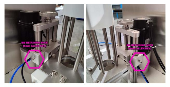
2.5.3 – Lower the apparatus to your desired can height. To test if the height is correct, push a can through with your hands. The can should not jam on the next spring apparatus (foam dampener).
