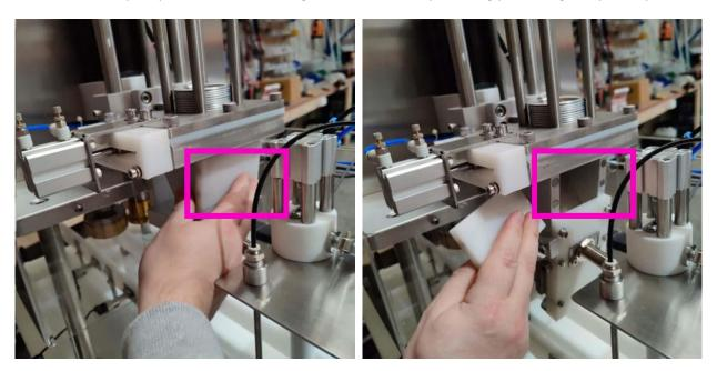
**2.5.2** – Unscrew / Loosen (to the point of falling off) the two retaining socket head screw caps on each side of the can lid dropper apparatus. With the 5mm Allen key in your toolkit.
