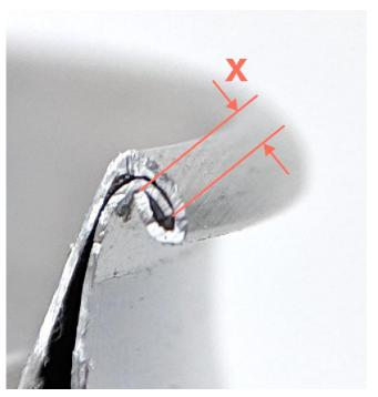
If you determine that the actual overlap between the can body and can end is less than 0.4mm following the first operation, make sure that your 1<sup>st</sup> operation roller is in the correct position.
