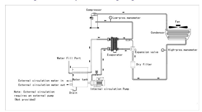
The Crystal8 industrial chiller uses a freon forced cooling method in which the glycol solution is constantly circulated through the plate heat exchanger and evaporator using the in-built pump. This in-built pump is only for internal circulation and does not circulate to external vessels. The plate heat exchanger takes advantage of shunt and counter current methods to maximise heat exchange efficiency.
