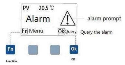
To determine the reason for the alarm press "Ok" to query the alarm. Then press "Ok" to reset the control panel.
