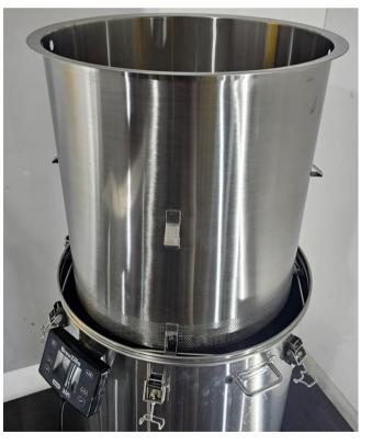
Once the malt pipe is suspended above the boiler and is securely supported by the halo ring then pour warm water (approximately 75-80°C) onto the top screen inside the malt pipe to rinse the grain of the majority of the remaining sugars. This process will probably require 40-50 Litres of water depending on your recipe and desired gravity that you are trying to achieve.
