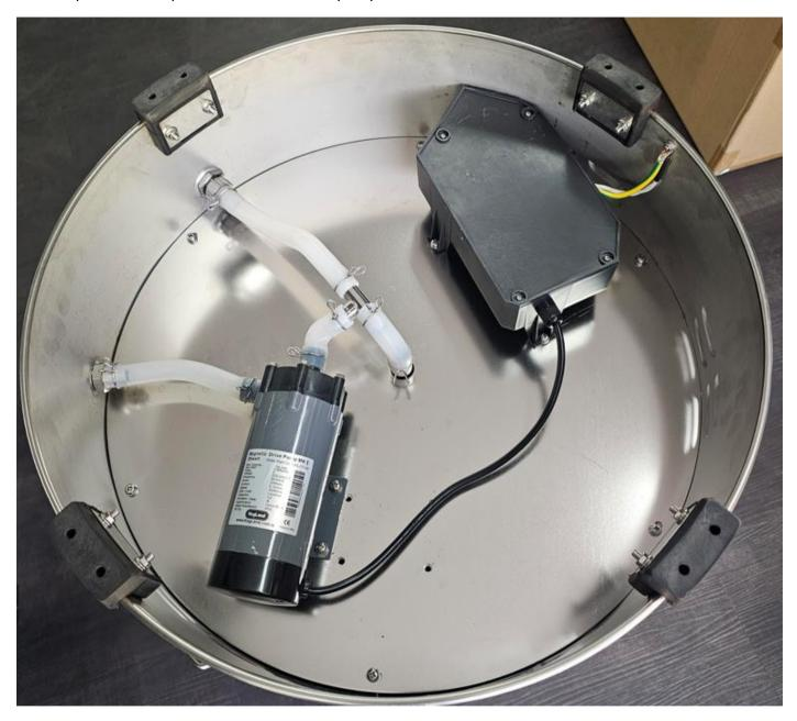
Make sure there are no kinks or twists in the silicone hosing which could impede the flow of liquid. If a kink is present then this may result in a pressure build up and the hose eventually splitting.
