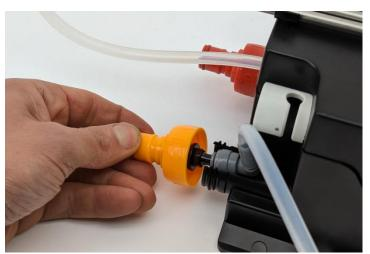
Screw the Ball Lock Post/Carbonation Cap onto the top of the machine as shown to the left.
