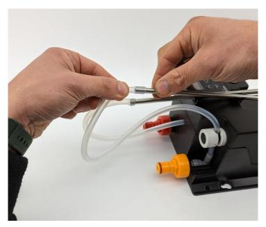
Push the silicone tube over the stainless tube and then clip the stainless tube into the front of the RAPT Can and Bottle Filler.
