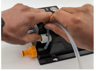
Using your thumb push down the black top of the pinch valve and this will open the pinch valve so you can slide the silicone tube into the pinch valve jaw as shown to the left.
