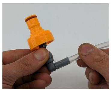
Fit the elbow to the barb of the Ball Lock Post/Carbonation Cap Barb. Then fit the silicone tube over the elbow as shown in the image to the left.
