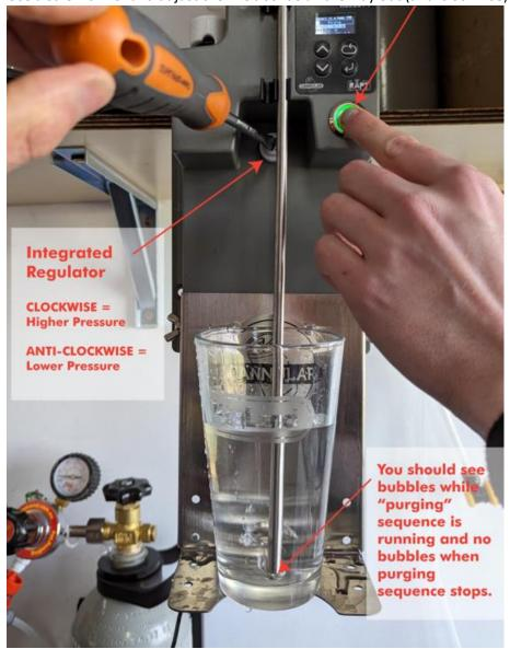
Place a large glass that is full of water into the machine. Press the start button then gradually turn the regulator adjustment screw clockwise until you see bubbles come out of the gas tube. Only a light flow of gas is required. Once you see vigorous bubbles in the water this will be sufficient.
