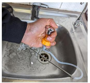
Hold the beer line and stainless tube up to your water tap and flush water through the tube.
