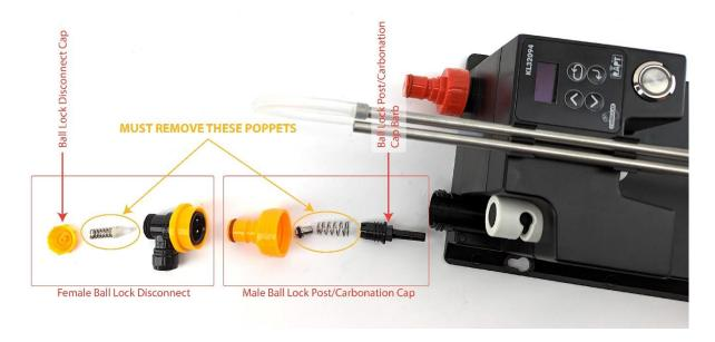
**NOTE:** Once you remove the poppets this quick connect is no longer a dry break connection. As a result, you will have to remember to disconnect the keg side before disconnecting the ball lock disconnect on the RAPT Can and Bottle Filler!
