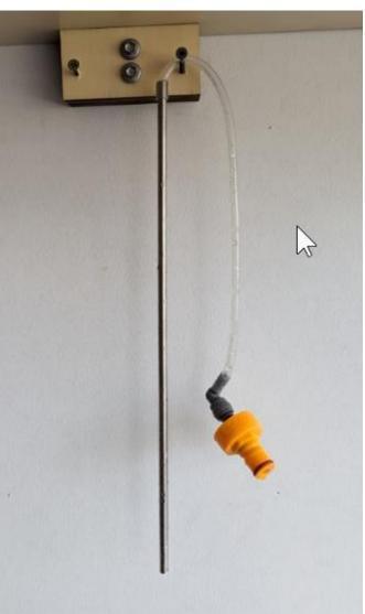
Hang the liquid tube assembly up on a hook so it can drain out completely.
