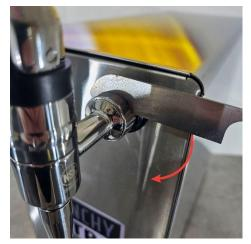
2. Unscrew the spout and remove the o-ring, aerator disc and regulation cone.
