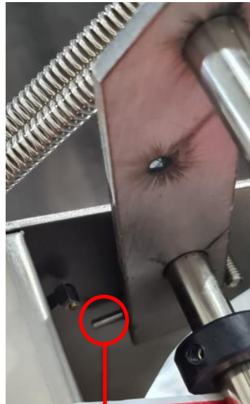
Adjust the amount of thread showing on the touch rod screw to alter when the microswitch is activated
