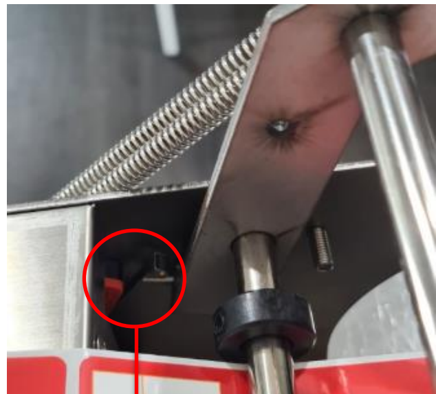
Adjust the amount of thread showing on the touch rod screw to alter when the microswitch is activated
