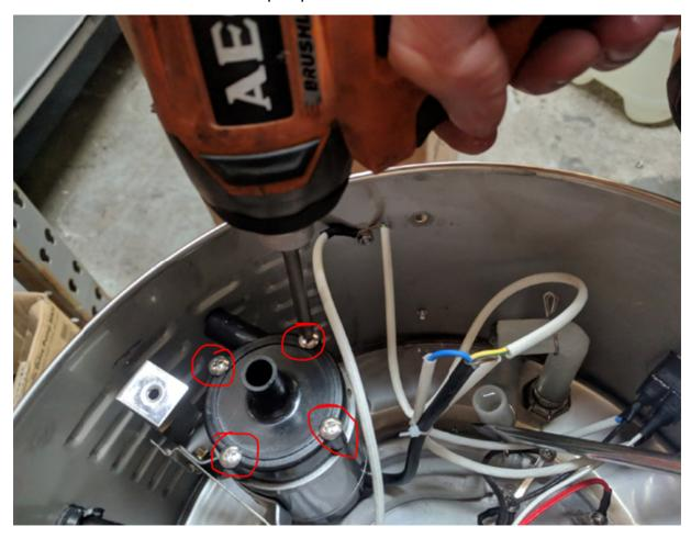
**Step 5**Check the pump head for debris and or solids that could be stuck in the pump head.
