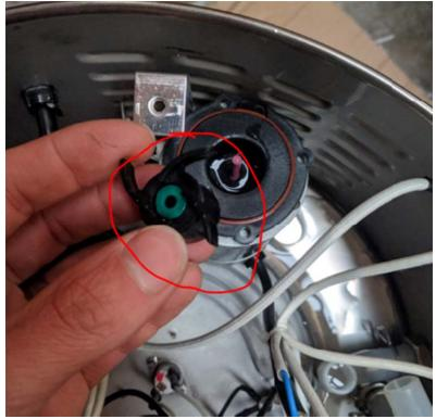
**Step 7**Look in the impeller housing and confirm no blockages are inside this side of the pump.
