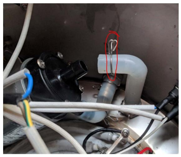
**Step 4**Remove the screws that hold the pump head on.
