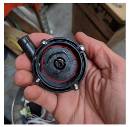
**Step 6**Check the impeller for damage or any blockage that could be stopping it from spinning.
