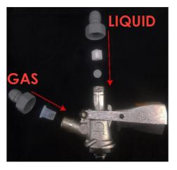
Insert check valves into keg coupler
