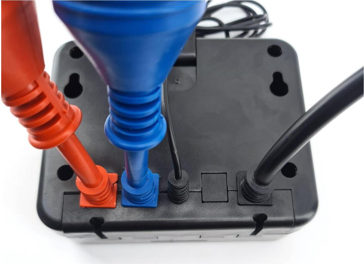
You can then custom design your own panel or cabinet to mount this temperature controller into with the outlets and wiring now exiting out the back of the controller allowing for a very neat mounting arrangement.
