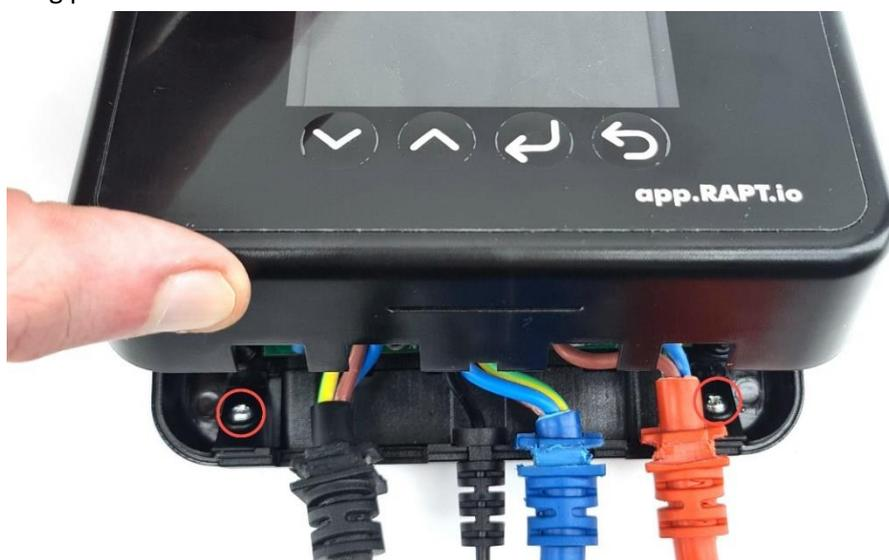
Move the cable glands to the back of the unit and secure in place with the slotted blanking plate, then secure the slotted blanking plate to the housing using the two screws. Then reassemble the front and back housings and secure with screws.
